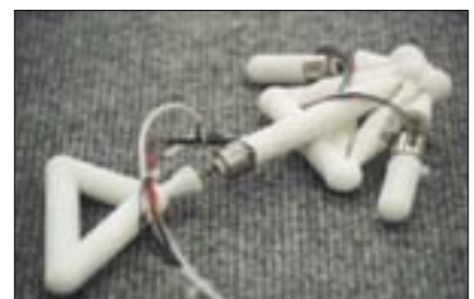
Figure 1: A picture of a Golem project's computer-designed evolvable robot, which pushes itself along the carpet using the piston at the center. (Source: The Golem Project at Brandeis University).
