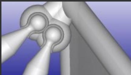
Close-up of a model of the evolved robot "Tetra" showing its ball and socket joints
