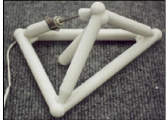
It takes a few days for the software to construct bodies-with-brains that best optimize the fitness function. Each run results in diverse locomotive mechanics and control circuits, all created without human knowledge. For example, one has a leg in the middle of its body to ratchet itself along the floor, while another swims the breaststroke on land.
