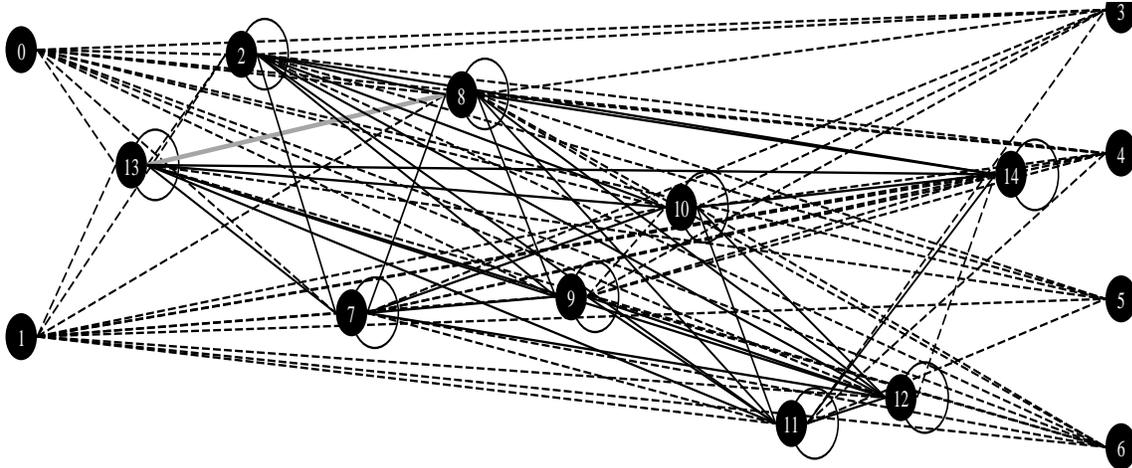
**Figure 2:** *The Tracker Task, first run. Network induced by GNARL after 2090 generations. Forward links are dashed; bidirectional links & loops are solid. The light gray connection between nodes 8 and 13 is the sole backlink. This network clears the trail in 319 epochs.*
