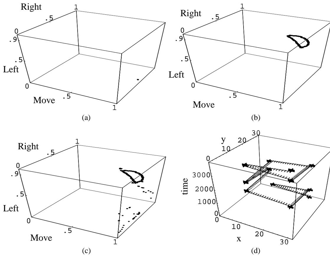
**Figure 4:** Limit behavior of the network of the second run. Graphs show the state of the output units Move, Right, Left. (a) Fixed point attractor that results for sequence of 500 “food” signals; (b) Limit cycle attractor that results when a sequence of 500 “no food” signals is given to network; (c) All states visited while traversing the trail; (d) The x position of the ant over time when run on an empty grid.
