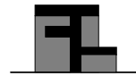
Figure 3. Shading Fitness Function. Only the gray region is shaded by the black structure.
