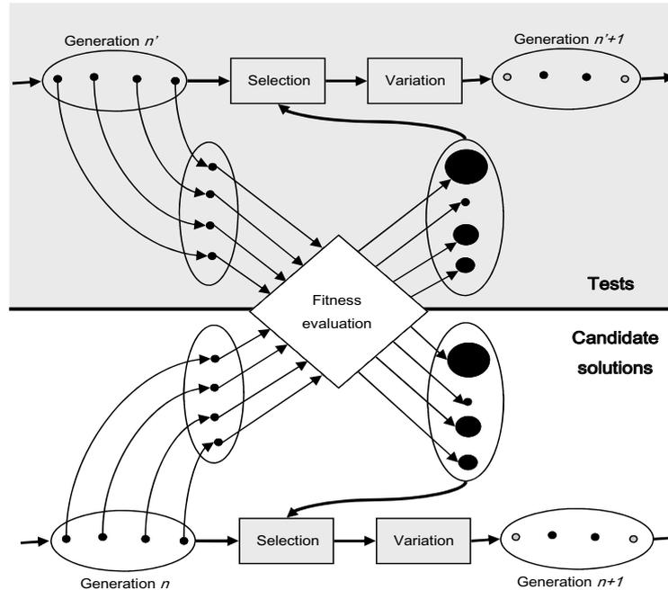
Figure 3.1: Schematic of the classic algorithmic configuration of a competitive coevolutionary algorithm.
