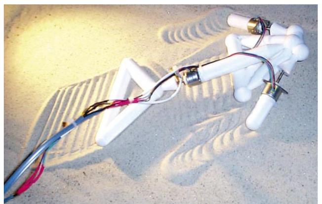
by symmetrical machines finding it easier to move in straight lines. This particular machine uses antiphase synchronization to move — while the upper two limbs push the machine forwards, the central body is retracted, and vice versa. Movies of this robot and others are available at <http://www.nature.com> as Supplementary Information<sup>1</sup>.
